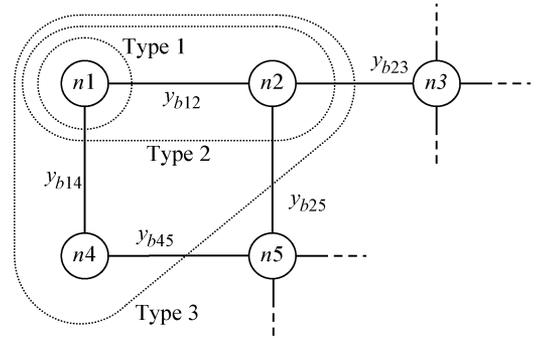
Fig. 4. Fencing constraints around the node  $n1$ .
